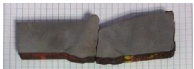
Figures 38a and b. Fatigue fracture from a notch due to lack of backing
