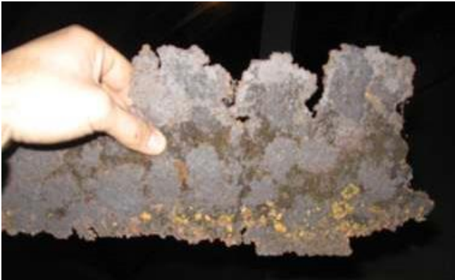
Figure 19a and b. Oxide thickness surface release due to the lack of weathering steels' own self-protection layer.
