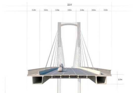
Figure 49. Current cross-section (5 lanes).
