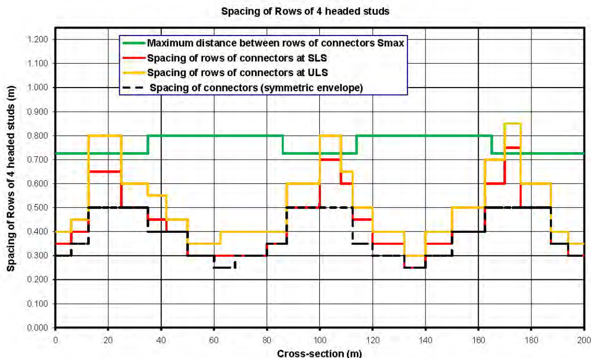
Fig. 6.29 Envelope of spacing of rows of 4 connectors after connection dimensioning
