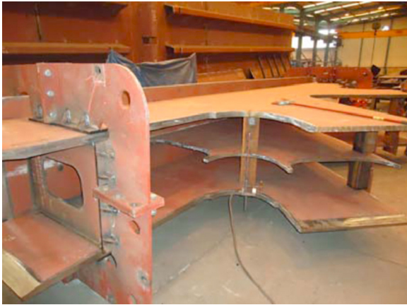
Figure 15. Manufacture of a recumbent node.
