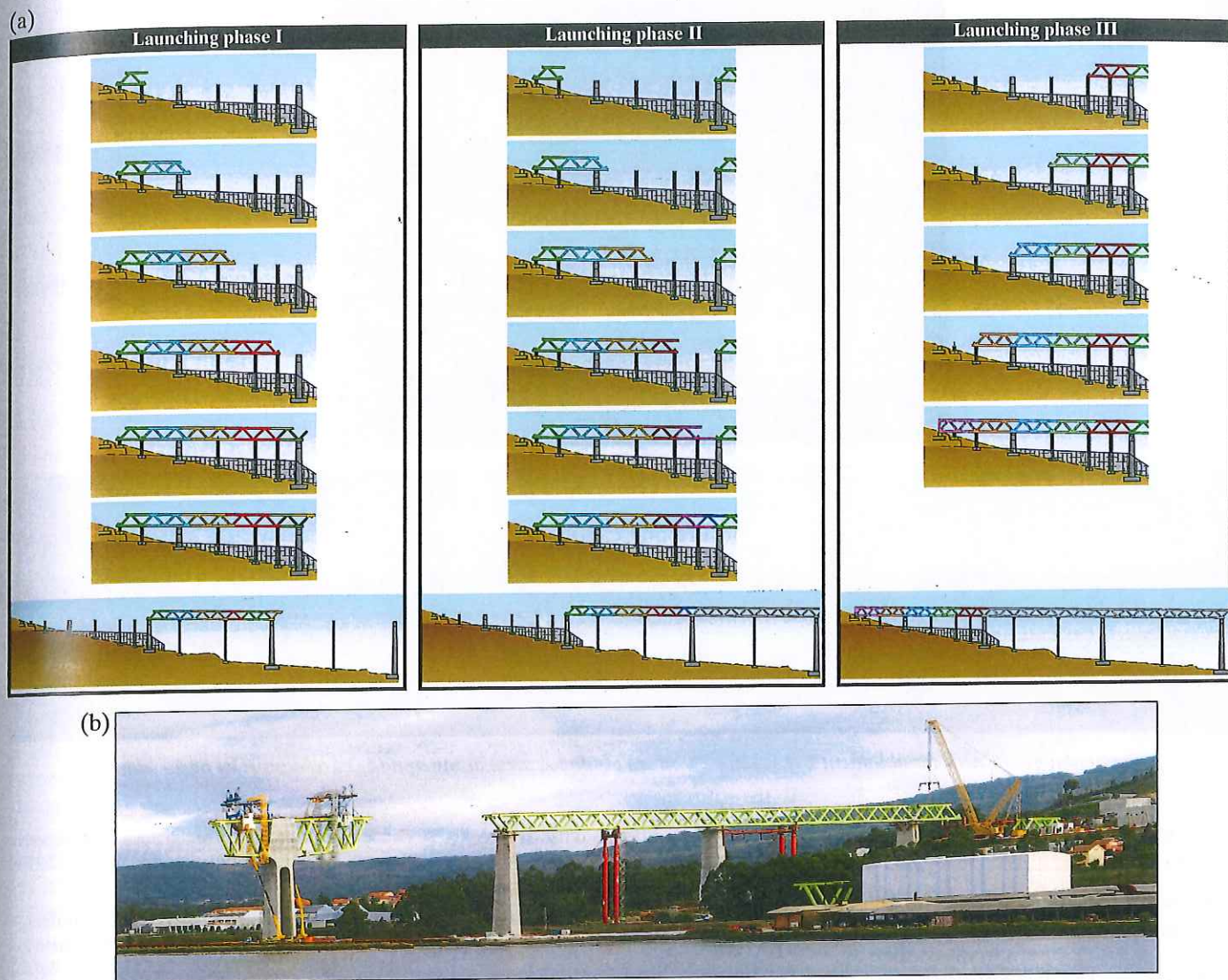
Fig. 10: (a) Scheme of the constructive procedure by launching in three phases and (b) picture of the current state of the works in December 2013 (launching phase III).
