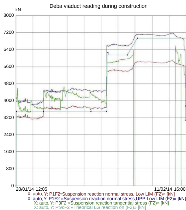
Figure 36. Reaction induced by the underslung scaffolding during the second phase of deck construction (with a 20 m cantilever and four concrete casting sub-phases).
